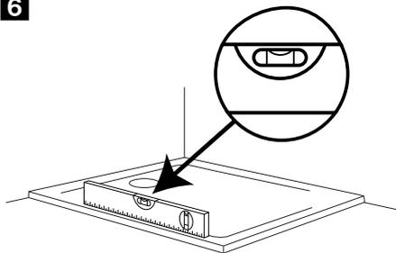
Place the shower tray **A** onto the wet adhesive ensuring that it is fully supported by the mix. Check the level of the top rims only as the shower tray has a built in fall for adequate drainage.
