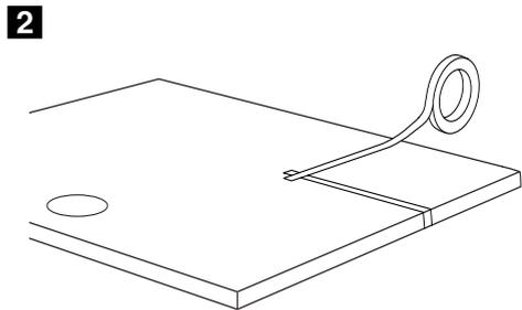
With the shower tray upside down, mark the lines to be cut on the back of the tray using masking tape or other suitable marking method.
