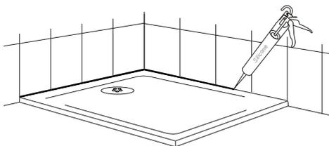
When the adhesive has set, remove any excess mix and masking tape, then make connection between the shower tray and waste piping. The shower tray and all connections **MUST** now be checked for water tightness, flow and adequate drainage over the entire area.
