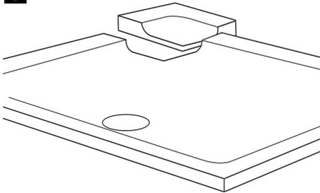
Taking care not to damage the visible surface, carefully remove any loose material and tidy the cut edge using 60 Grit (or similar grade) sand paper.
