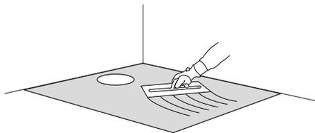
Use installation compound adhesive or a suitable contact adhesive to cover the full area under the shower tray. Apply or trowel to a thickness suitable to allow full adhesive support of the shower tray.
