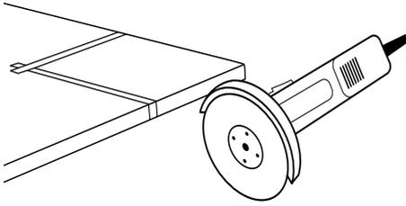
Carefully cut the marked area from the shower tray using a minimum of a four inch (approx 102mm) diamond blade (suitable for cutting stone) on an angle grinder or other suitable cutting tool.
