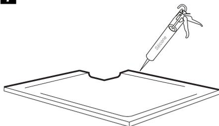
Before fitting, apply copious amounts of silicone to the edges of the shower tray **A** against all wall contact points.
