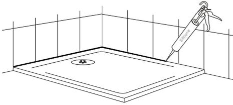
When the adhesive has set, remove any excess mix and masking tape then make connection between the shower tray and waste pipe. The shower tray and all connections **MUST** now be checked for water tightness, flow and adequate drainage over the entire area.
