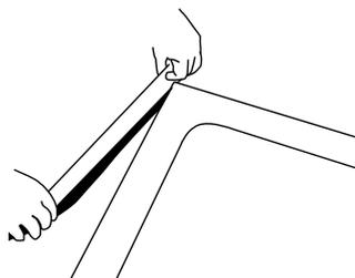
Attach to the edge of the shower tray so that it is square and the edge protrudes at least 20mm above the edge of the tray.
