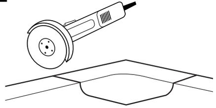
It may be necessary to turn the shower tray over to obtain a through cut on the thicker section of the periphery of the tray, depending on the size of the blade being used.
