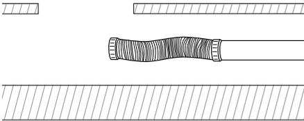
Remove the plywood and install the waste outlet pipe in the cavity in accordance with building regulations.
